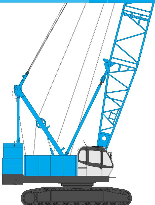
Max. Lifting Capacity: 100 t x 3.8 m Max. Crane Boom Length: 62.6 m
